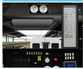
Follow the driver's instruction to "TOMARE(stop)" and bring the train to a stop 3 meters before the coupling position.
