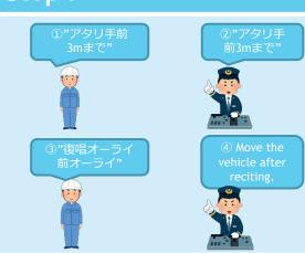
Recite the instructions of the connecting operator and move the vehicle to 3m before the connecting position.
