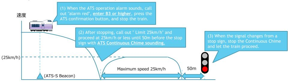
When the signal indicates something other than a stop, the Continuous Chime will stop, and the train will return to normal operation.
