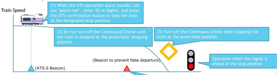
The emergency brake is automatically applied when the train passes a beacon to prevent false departure after a certain period has elapsed since the train entered the station.
