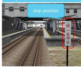
Stop the vehicle at the target stopping position and load the connecting operator.
