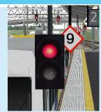
Indicates that the movement of the train/car is prohibited due to merging, splitting or inspection.
